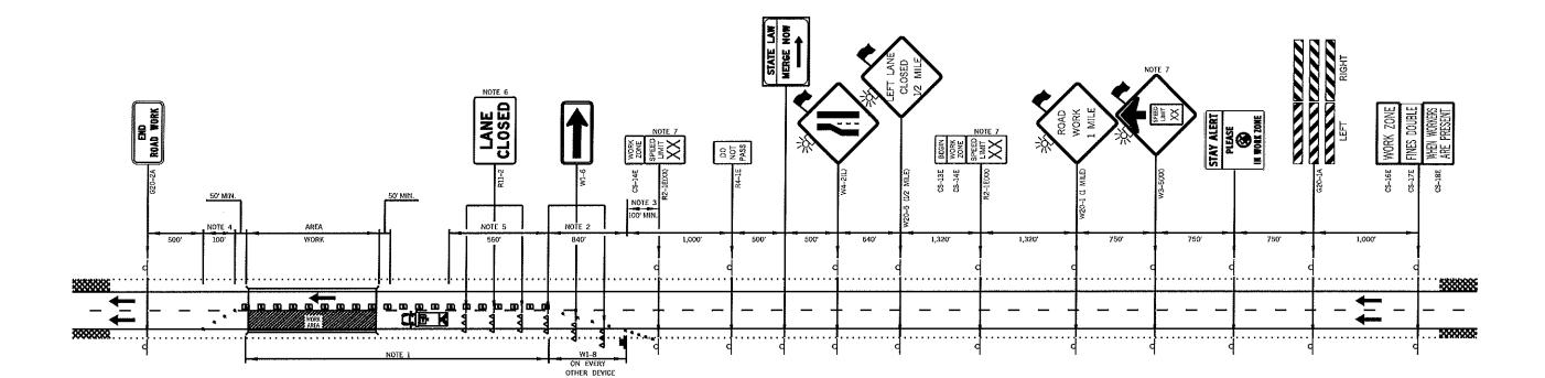
MAXIMUM SPACING BETWEEN CHANNELIZING DEVICES (FEET) SHALL BE TWICE THE POSTED SPEED LIMIT (M.P.H.) WITH THE FOLLOWING EXCEPTIONS. SPACING SHALL NOT EXCEED 50 FEET FOR CONES OR TUBE CHANNELIZERS. SPACING SHALL NOT EXCEED 75 FEET FOR CHANNELIZER CONES.SPACING SHALL NOT EXCEED 100 FEET FOR TYPE II BARRICADES, VERTICAL PANELS OR DRUMS.
